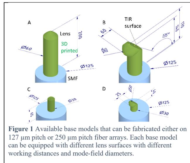
**Figure 1** Available base models that can be fabricated either on 127  $\mu\text{m}$  pitch or 250  $\mu\text{m}$  pitch fiber arrays. Each base model can be equipped with different lens surfaces with different working distances and mode-field diameters.
